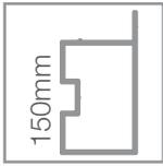
The optional bolster is available to raise the ceiling height by 150mm when required. With the use of the bolster spans of up to 6000mm can be achieved for large bi-folding doors.
